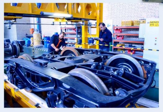
The Y25-Lsd1 is a standard UIC-ORE bogie, designed for freight wagons running with speeds of up to 120km/h, the gauge of 1,435mm and the load of 22.5t. The bogie consists of wheel set, axle box, suspension, bogie frame, bogie brake, load proportional device and etc.
